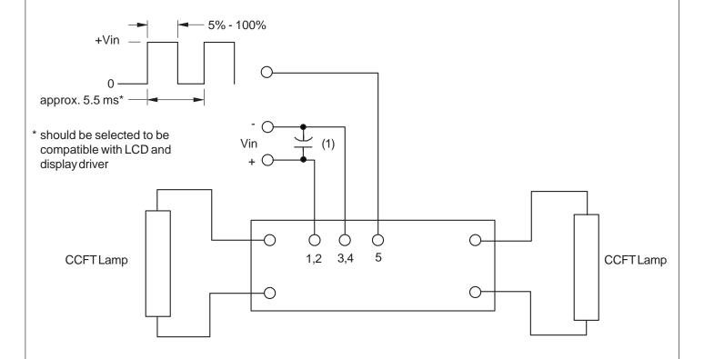
Pulse-Width Modulation Controlled
