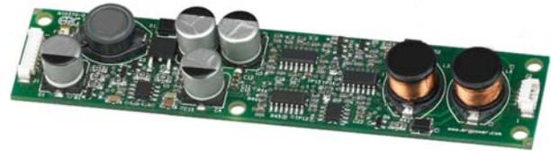
Figure 7A -- Example of PWM voltage boost with multiple hysteretic current sources. (SFDC series from ERG)
